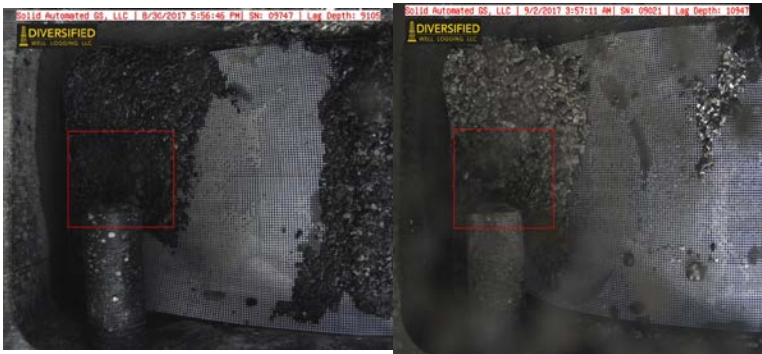
Fig 5. Sample photograph of collected drill cuttings in the ARM, Automated Remote Mudlogger
