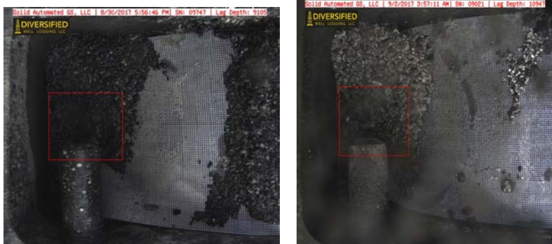
Fig 5. Sample photograph of collected drill cuttings in the ARM, Automated Remote Mudlogger
