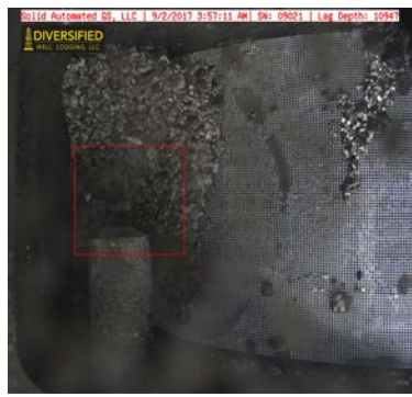
Fig 5. Sample photograph of collected drill cuttings in the ARM, Automated Remote Mudlogger
