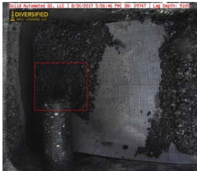
Fig 5. Sample photograph of collected drill cuttings in the ARM, Automated Remote Mudlogger
