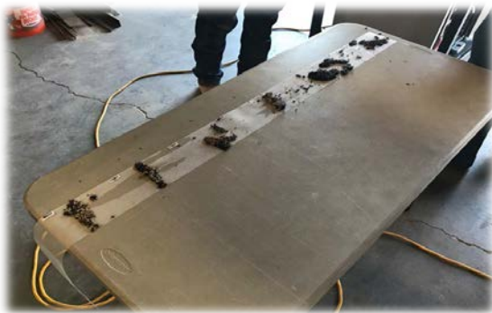
Fig 6 system collected 447 samples with 349 samples of 10gms or greater. A 78% success rate. ROP -25/hr. in the final 2000’ created a low available cuttings environment, and reduced success rate. The Compositional data of the rocks collected by the ARM and the mudloggers manually showed a general broad agreement. Differences observed can be attributed to spot sample (ARM) versus wider intervals collected manually.
